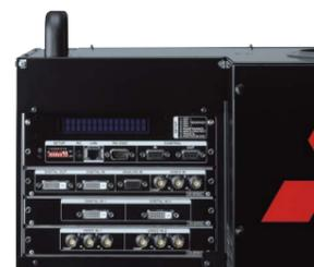
The number of input boards has been increased for compatibility with a wider range of input signals. Compatibility with input resolution has also been increased, now including up to WUXGA (1920x1200).
