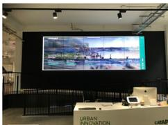
After evaluation of technologies for the reception a flat panel solution was chosen to fill the rear wall. The solution provided a true resolution of 9,600 by 3,240 pixels which delivered a stunning very resolution image, 4K+. Control was done using Harps Commandant window manager Application.
